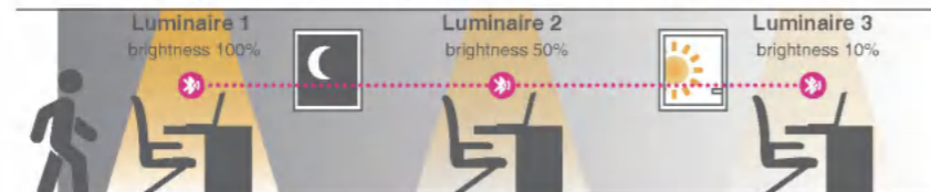
Schematic diagram 3 - Luminaires group, daylight detection & compensation
